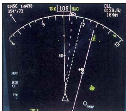
Taken at FL 370, return at 2 o'clock and 20 miles appears weak because the bottom of the beam is approaching the radar top. Note the tilt is set to zero degrees, 80-mile range selected, with no ground returns displayed.
